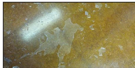
The process of the coating separating from the substrate in either large or small sections or a flaking off of the coating.
