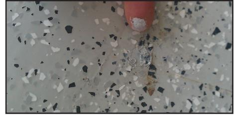
Surfaces or areas of the surface that have not completely cured. Product remains in a liquid, tacky state.
