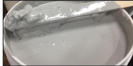
Lumps (crystals) floating in liquids, cloudy appearance, or even a completely solid mass can all be evidence of epoxy crystallization.
