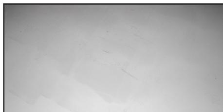
The process of having light and dark streaks visually observed when applying a coating to the substrate.
