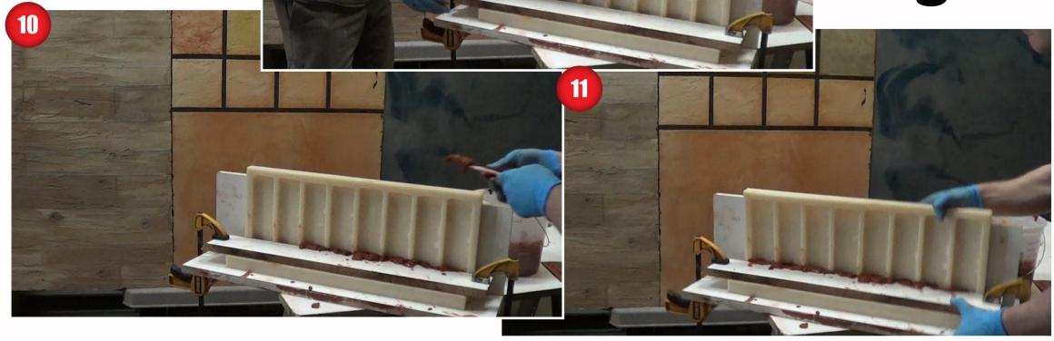
Flip the <u>mold</u> over when the concrete is no longer flowing, and wont spill out. Fill the other side of the mold with concrete
