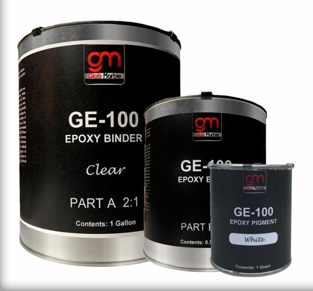
Our GE-100 Epoxy along with its solid pigment can be used as a primer coat and has a coverage of approximately 100 square feet per gallon. Primer coats are important for masking the color of the concrete floor, and the color of the primer should match the color of your metallics. White for light colors, black with dark.
