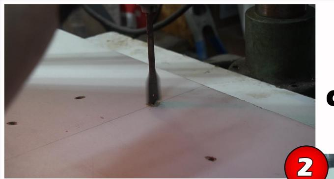
A spade bit is used to drill counterbore holes for the bolts
