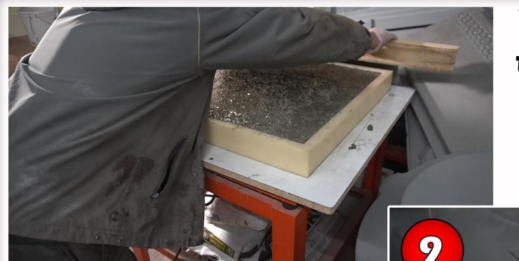
You can then screed the top of your mold to remove any concrete above the form walls.
