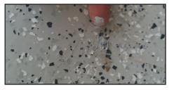
Surfaces or areas of the surface that have not completely cured. Product remains in a liquid, tacky state.
